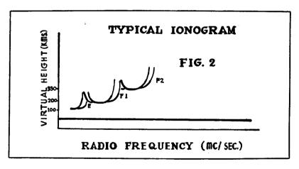
Normally the echoes present a sharp trace corresponding to each of the layers that are present at the time. At the horizontal part of the trace the minimum height for the layer can be read off by comparison with the height markers. As one follows with the eye the echo trace of a particular layer from the leveling-off point in the direction of the higher frequencies, he observes that the apparent height increases and the curve rises until it shoots vertically upward. The
